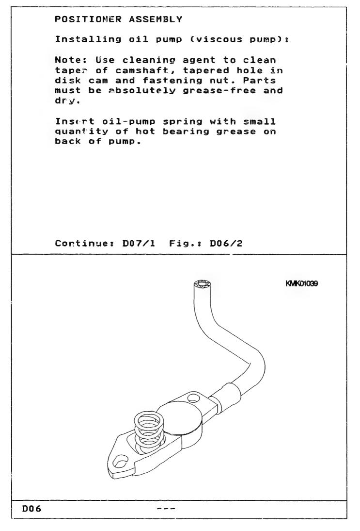
Installing oil pump (viscous pump):
